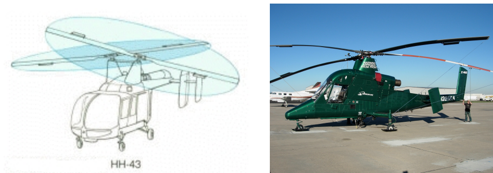
Figure 3.4: Sketch of an intermeshing helicopter (left) [1] and an image of a Kaman K-1200 (right) [13].
